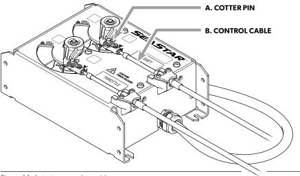
Figure 4-1. Actuator manual override.
