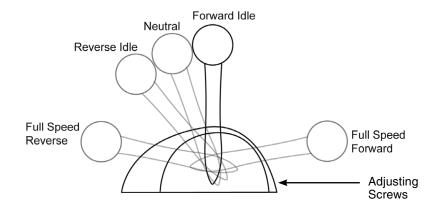
Figure 3-8. Control Head lever positions.
